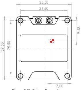
Figure 2.31: Ellipse-D top view
