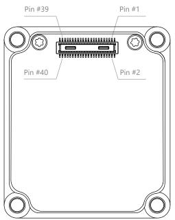
Figure 2.36: OEM units connector orientation (bottom view)
