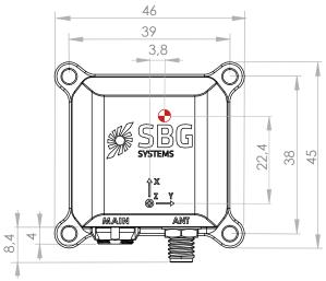
Figure 2.15: Ellipse-D top view
