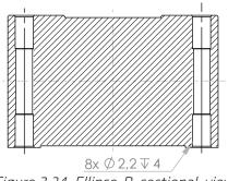
Figure 2.34: Ellipse-D sectional view
