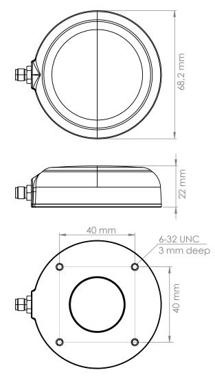
Figure 5.13: Tallysman 7972 mechanical drawing
