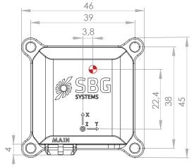
Figure 2.3: Ellipse-A top view
