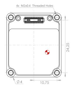
Figure 2.32: Ellipse-D Bottom view
